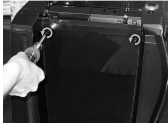
Open the two oval-head screws with the aid of the included oval-head bit insert
