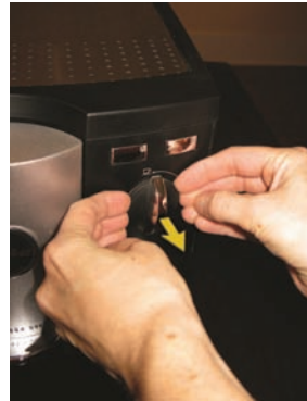
Remove the steam dial by pulling it straight out.
