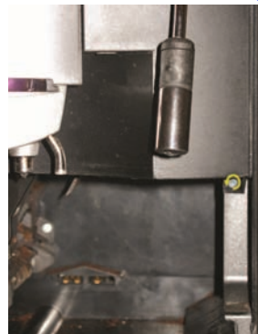
Unscrew the screw marked with the arrow. Carefully lift up the two clips marked by the blue arrows and pull the steam assembly in the direction of the yellow arrow so that it unlatches.
