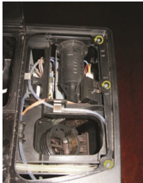
Swing up the cup warmer plate and remove it. Then remove the three screws marked with arrows.
