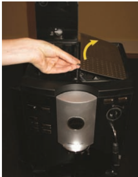
Swing up the cup warmer plate and remove it. Then remove the three screws marked with arrows.
